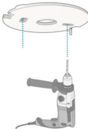
**EN** Position the mounting plate in the final location (instructions on pages 4-5) and mark the holes. Drill the holes and insert the plugs provided.
