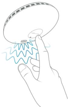
**EN** You should test the smoke detector every month to ensure that it is properly installed and working correctly. You can carry out the test directly on the detector by pressing the central button for three seconds.
