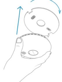
**EN** Then fix the detector to the plate by turning until it locks in place.
